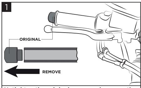
**Untighten the original screw and remove the counterweight.**
