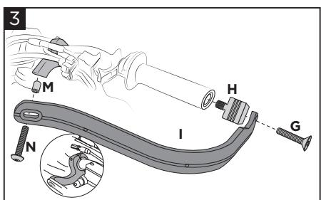
**Fix the bar (I) to the handlebar using the spacer (H) and the screw (G) as shown in the figure. Fix the bar to the bracket using the screw (N) and the bushing (M).**
