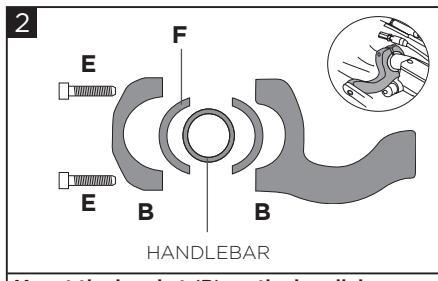
**Mount the bracket (B) on the handlebar using screws (E) and use the spacers (F).**
