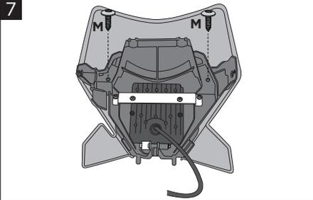
**Fix the internal frame in the mask using the original screws (M).**
