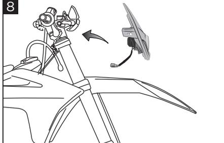
**Remount the headlight mask by connecting the connector.**
