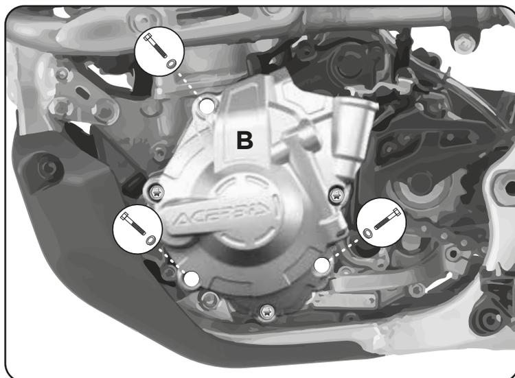
**Remove 3 OEM ignition cover bolts exactly as indicated in the image above. Attach the X-Power ignition cover with the remaining 3 (C) bushings and the 3 stock ignition cover bolts and tighten to the OEM torque settings in the owners manual.**
